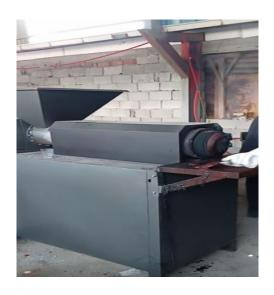
The melted mixture is then placed in a press mold, where it is pressed and a finished tile is obtained.
