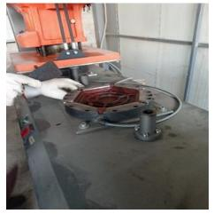
At the end of the process, it is placed into cold water to keep its shape.
